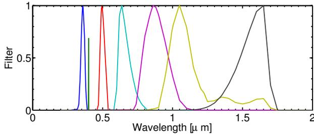
**Fig. 1** Transmission functions  $T_f$  for the DIFOS experiment (Link). The filter at 400 nm corresponds to the SPM instrument installed onboard the SOHO observatory.
