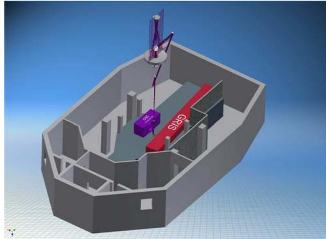
**Fig. 3** (online colour at: [www.an-journal.org](http://www.an-journal.org)) Physical location of Gregor@night. It is the smaller box with respect to the GRIS spectrograph whose optical table is shared. The telescope optical beam is shown in the night-time configuration, i.e. the F3  $f/41$  focus is occupied without the AO beam and without the image derotator but with the spectrograph fore optics. The total system until the spectrograph slit contains of 10 mirrors.
