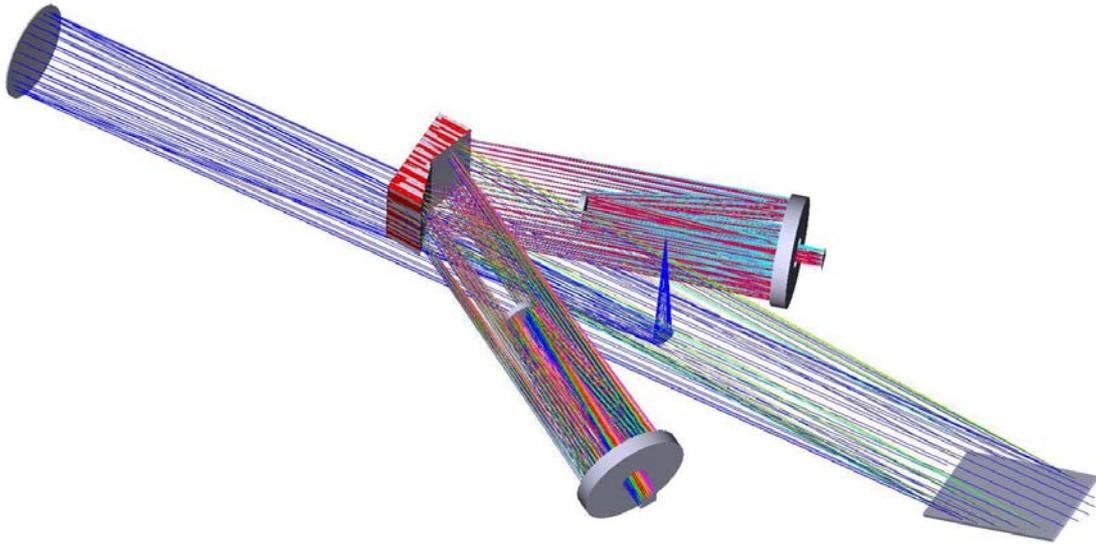
**Fig. 2** (online colour at: [www.an-journal.org](http://www.an-journal.org)) Zemax design of the refurbished SoFINE spectrograph, now called Gregor@night. The light injection is in the middle of the figure and from the “top” just before a 90-degree bent of the beam. The grating is to the right and the collimator to the left side of the picture. The cross disperser prism is seen in the middle in two positions feeding either one of two reflective cameras.
