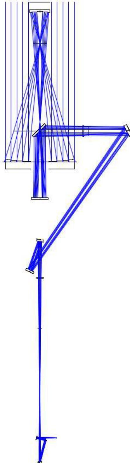
**Fig. 5** (online colour at: [www.an-journal.org](http://www.an-journal.org)) Zemax design of the full light path until the spectrograph entrance. The fore optics are the last three mirrors at the bottom, two of them off-axis parabola and one a flat (shown in detail in Fig. 4a).
