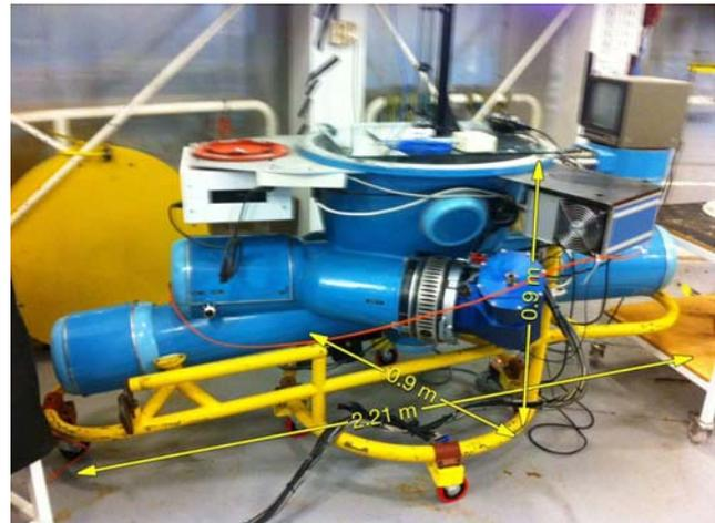
**Fig. 1** (online colour at: [www.an-journal.org](http://www.an-journal.org)) The SoFINE spectrograph after dismounting from the Cassegrain focus of the NOT. The overall dimensions in meters are indicated. The instrument is shown on its trolley in zenith-pointing position with the circular telescope flange at the top. This spectrograph will be the base of the new Gregor@night instrument.
