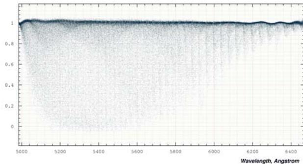
**Fig. 6** (online colour at: [www.an-journal.org](http://www.an-journal.org)) Full spectral range of the iodine-gas absorption for cell AS#3 in Gregor@night. The useful wavelength range with absorption lines is 500–630 nm.
