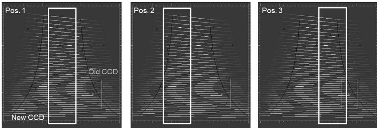
**Fig. 7** Echelle coverage for three different grating tilts dubbed Position 1, 2, and 3 (from left to right). Shown is the size of the new e2v 2k×2k CCD with 13.5 μm pixels (large white box) compared to the old CCD (EEV 1200×330 pixels). Note that the scales for the two axes are not identical and thus the squared CCD appears as an elongated box.
